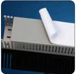
Flexible, double scoreline for fast and easy modification. No cutter needed for first scoreline. Flush/Burr free break. Second scoreline easily removed with Triton side wall cutter.
